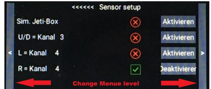
The buttons of the JetiBOX are controlled via 2 or 3 servo channels. Channel 3 is preset for the UP and DOWN buttons, and channel 4 for left and right.
