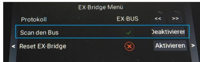
You can follow the scanning process in the status display. Since some Jeti-EX sensors are only approx. 20sec. Long send the names of the values, the sensor should be plugged in immediately after the start of the scan. When the scan is complete, the following status message appears. (if you miss some values, start the scan twice)
