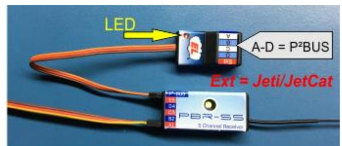
If the receiver is switched on, a red LED lights up in the Tele-Bridge.
